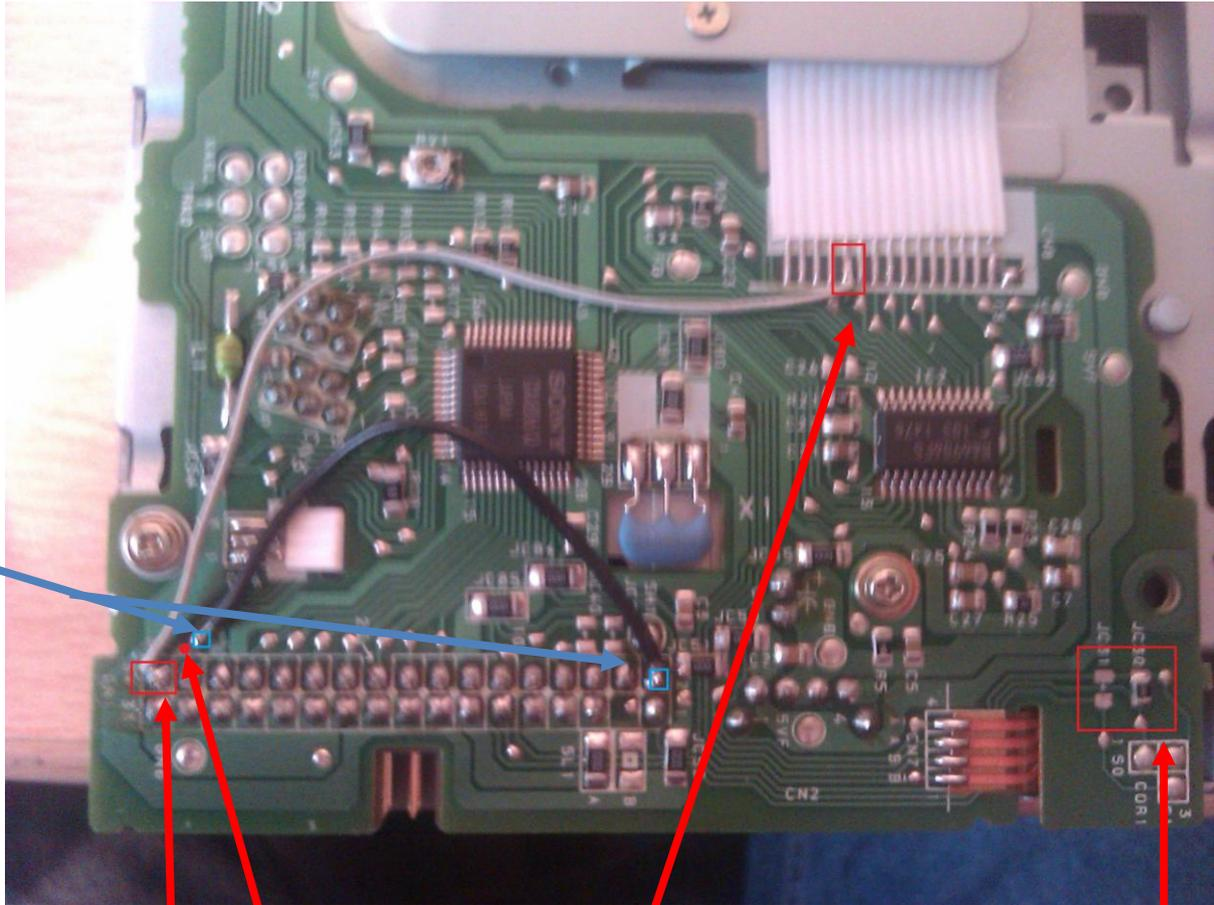
Cable track broken from solder joint to pin 34
