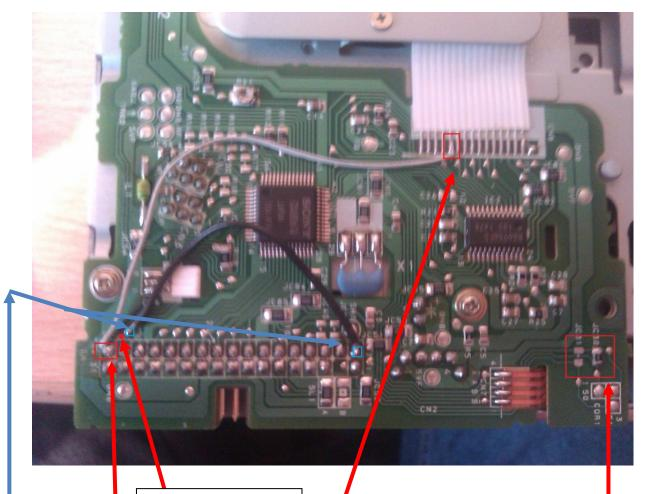
Cable track broken from solder joint to pin 34
